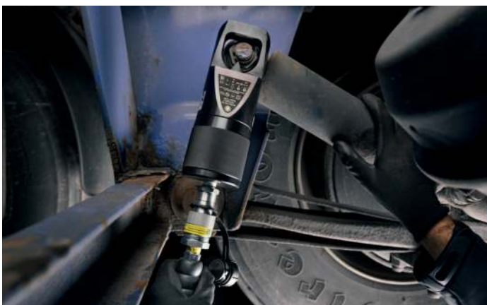
The single-edged, pump-hydraulic nut splitter Y-57 splitting a nut on a vehicle
