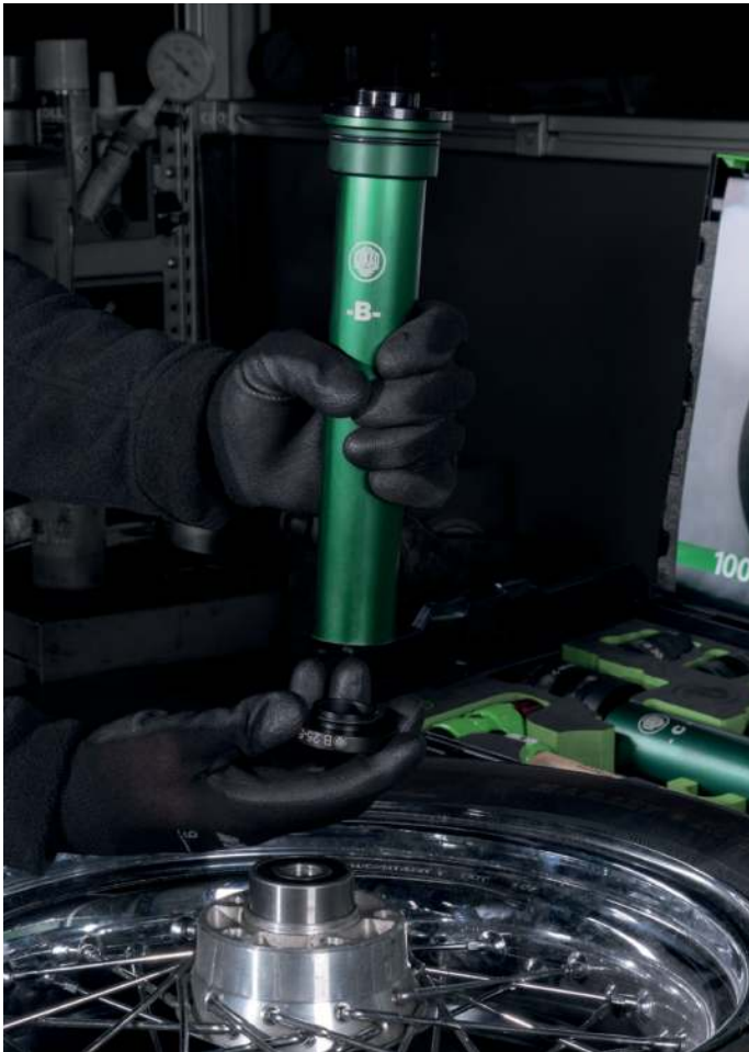
Inserting the matching impact ring into the impact tube when using a K-71 set
