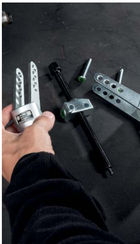
Reassembling the individual components and reversing the jaws
