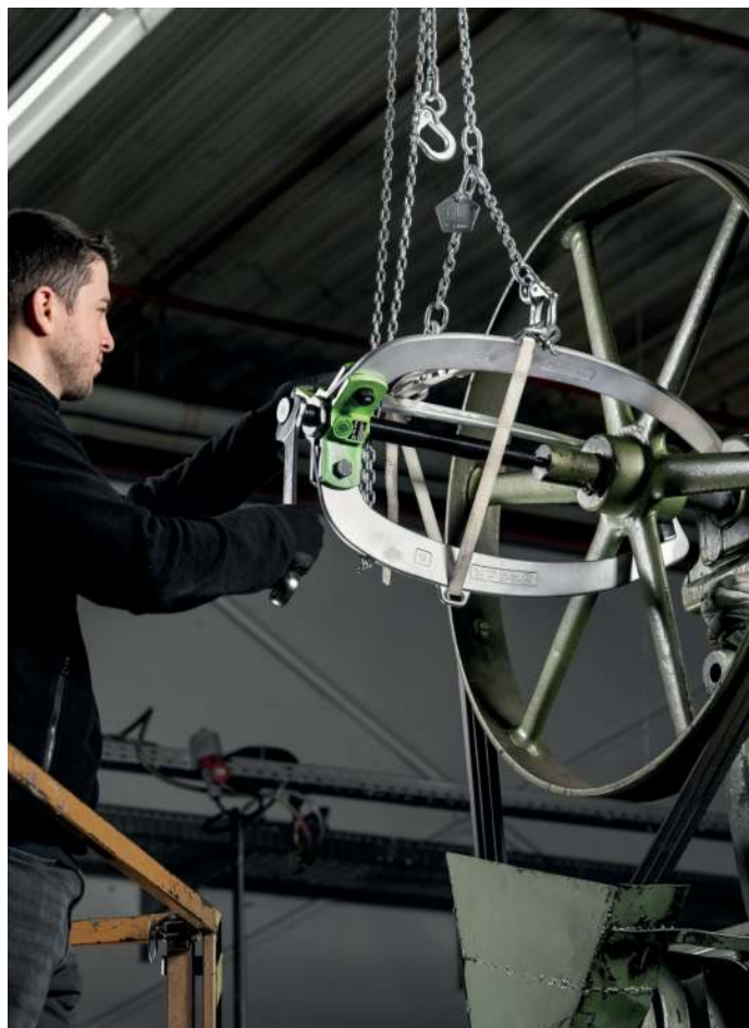
An additional lashing strap secures the jaws
