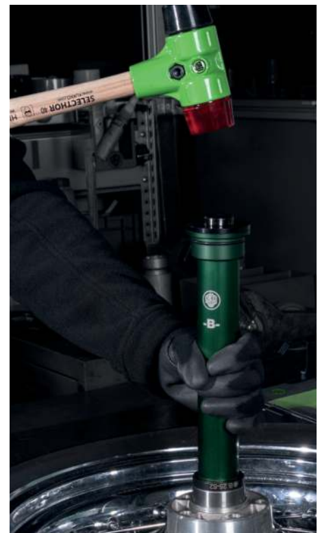
Ball bearing installation with the K-71-L
