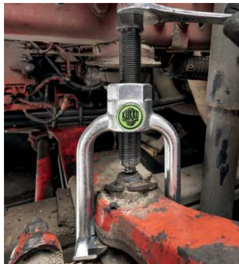
The ball joint puller 128-60 in use pressing out a tie rod end on a tie rod in a workshop
