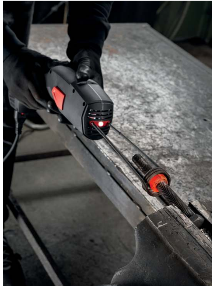
Heating a nut with a heating coil
