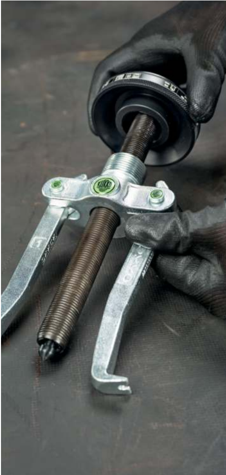
Fitting the clamping cone rotated by 180
