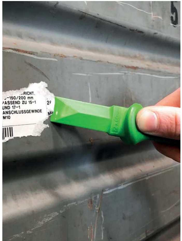
A soft scraper from series 2200 gently removing a product label
