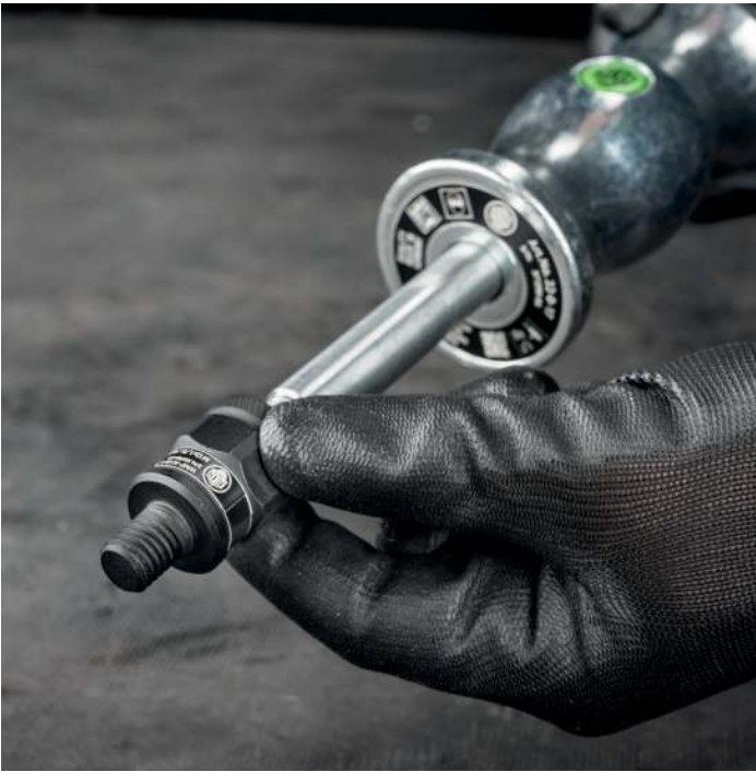
By combining a thread adapter with a sliding hammer (series 22-0+), a component with an internal thread can be pulled out particularly gently using high tensile force.
