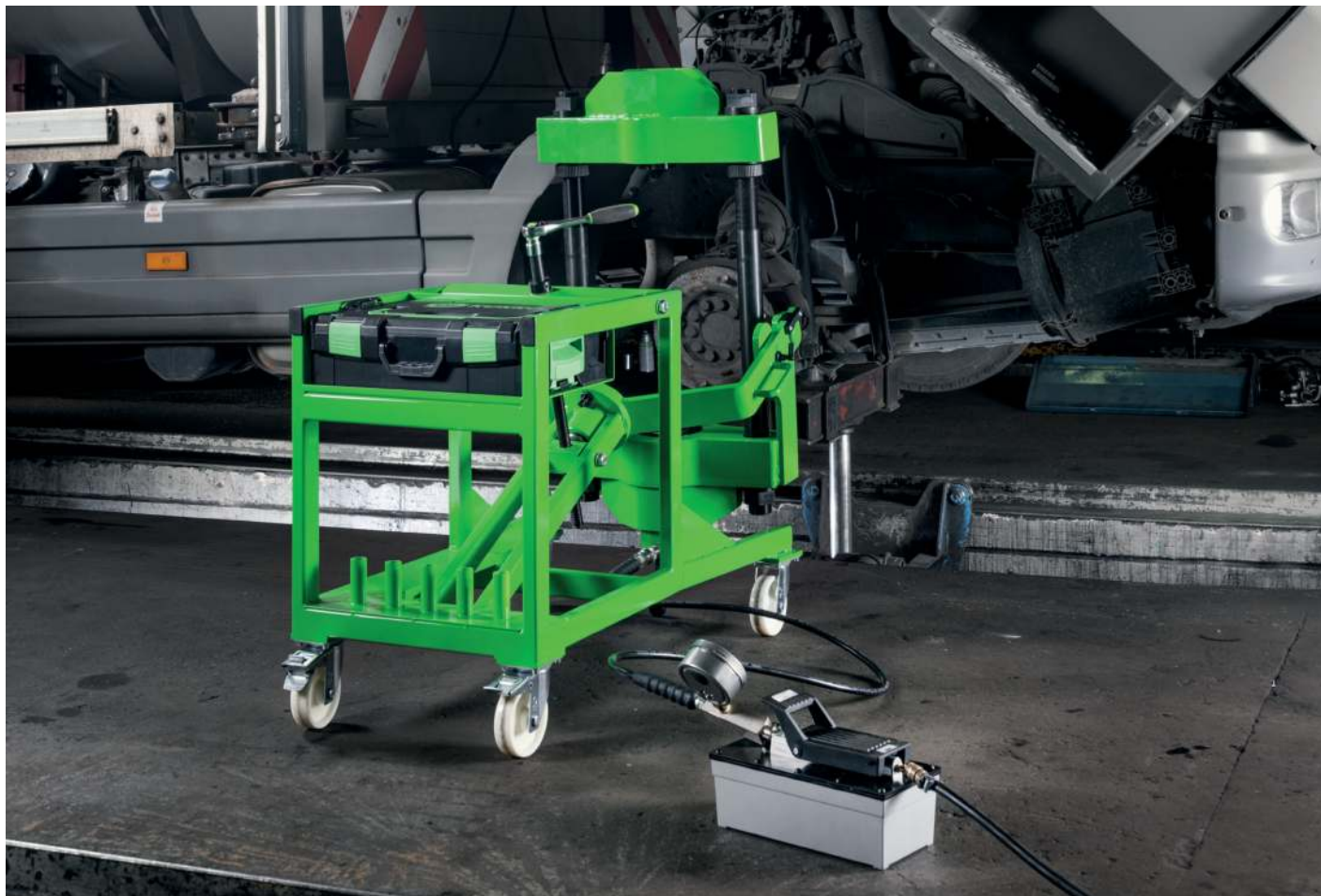
The hydraulic king pin press "AXLE"Y-AP-75 is ready for use on a truck
