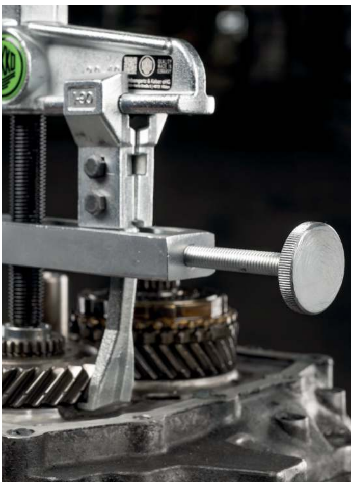
The clamp presses the jaws to the part to be pulled off
