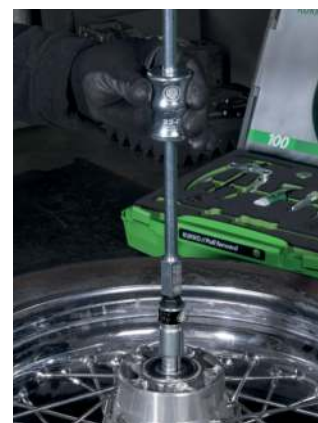
Internal extractor series 21 with sliding hammer
