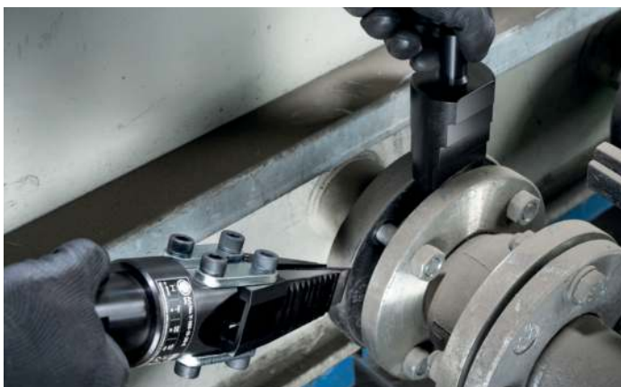
A hydraulic spreader of the Y-165 series with a safety block that holds the flanges in the spread position.
