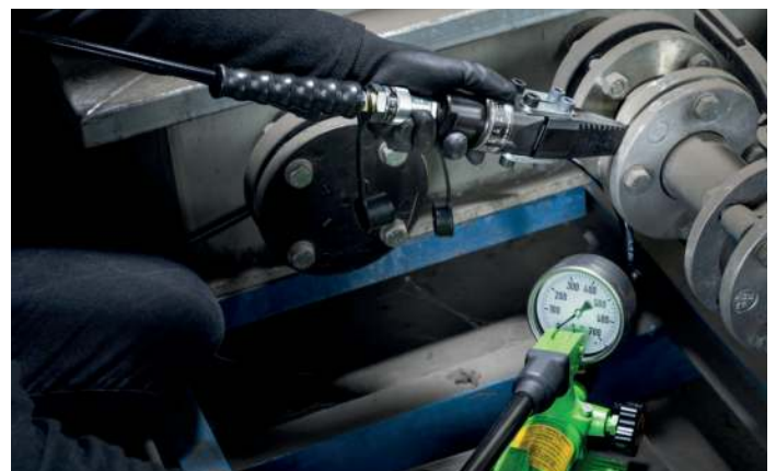
The hydraulic spreader of the Y-165 series with hydraulic hand pump when spreading a flange connection.
