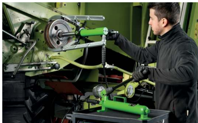
Pulling of a pulley from a combine harvester with the Y18-208
