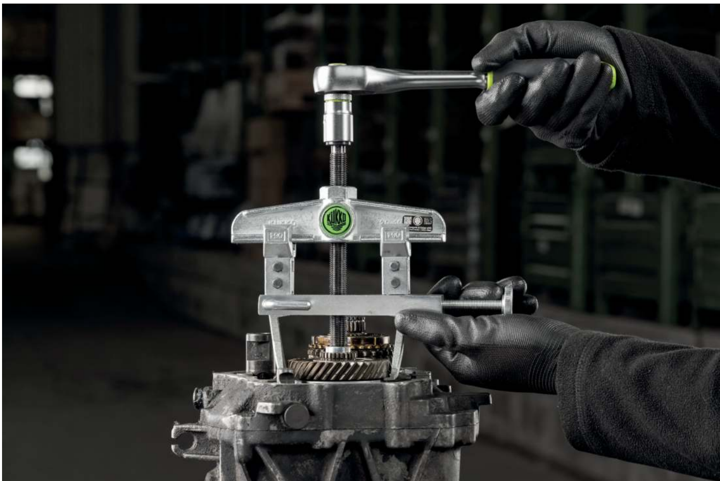
Pulling a gear wheel with the 20-10-V
