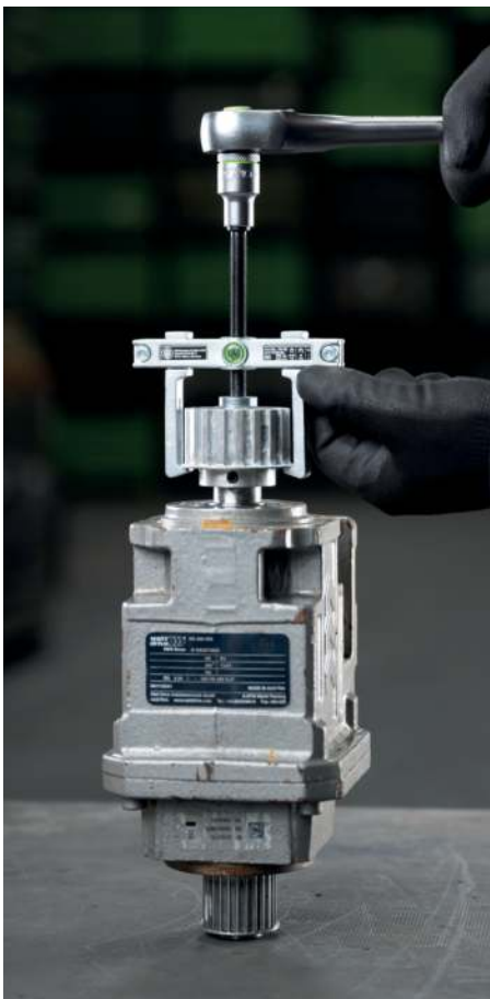
Pulling a pulley from a machine gearbox with the 110-02
