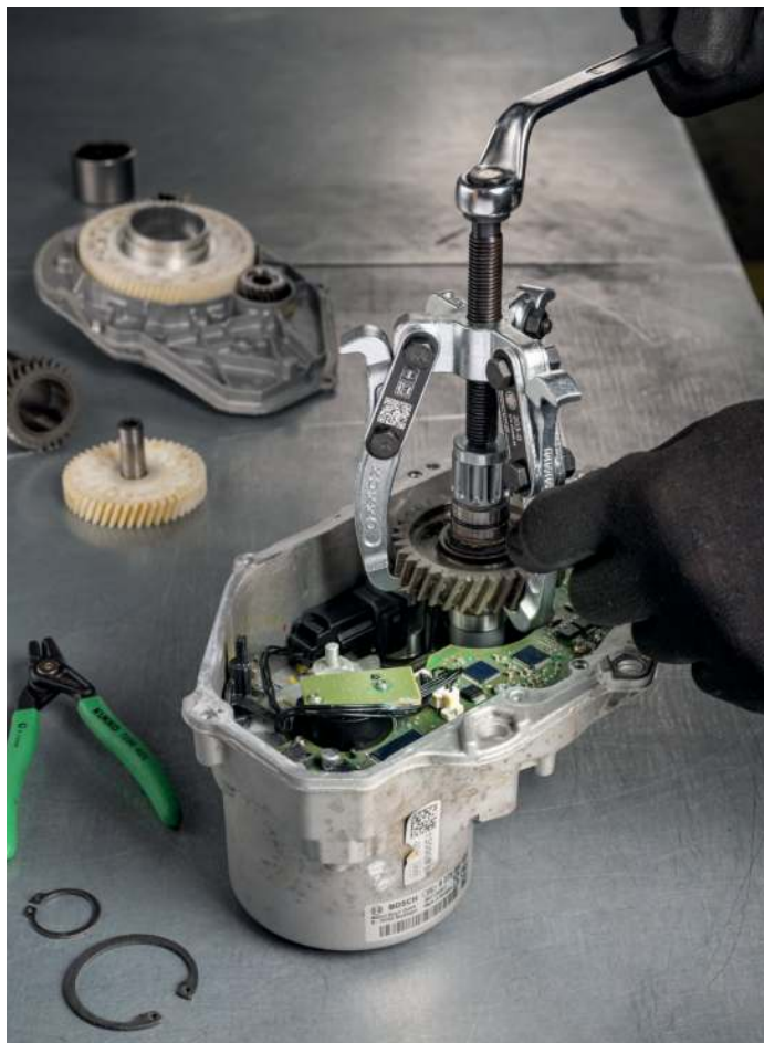
3-jaw puller with crossbar when removing a gear from an electric motor.
