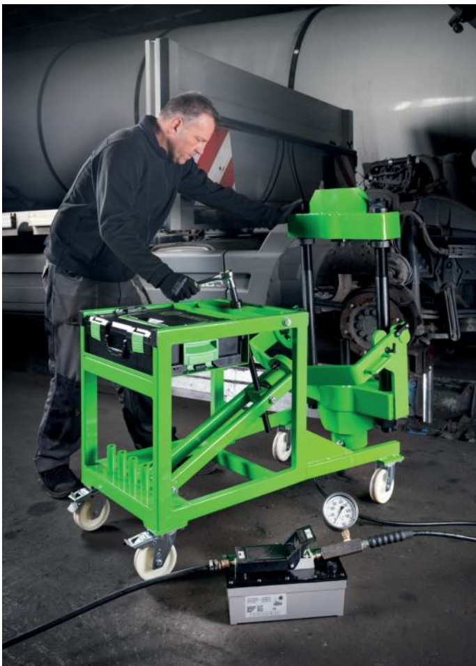
The hydraulic knuckle pin press "AXLE"Y-AP-75 is adjusted with a ratchet
