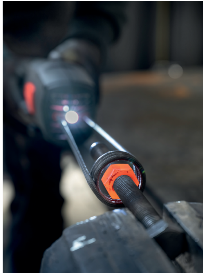
If the device's internal temperature is too high, the heating process is automatically stopped.
