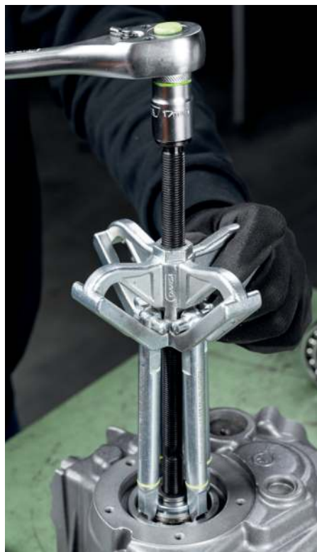
Ball bearing removal with the 70-0
