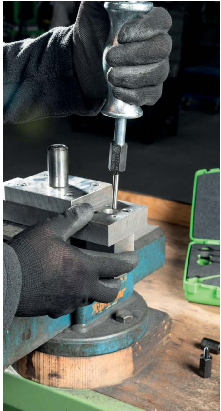
Internal extraction of a dowel pin with a sliding hammer and thread adapter
