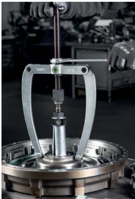
Extracting a ball bearing using a counter stay and thread adapter
