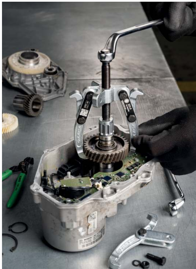
Thanks to the crossbar, the 203-0 can also be used for 2-jaw pulling after a quick conversion.
