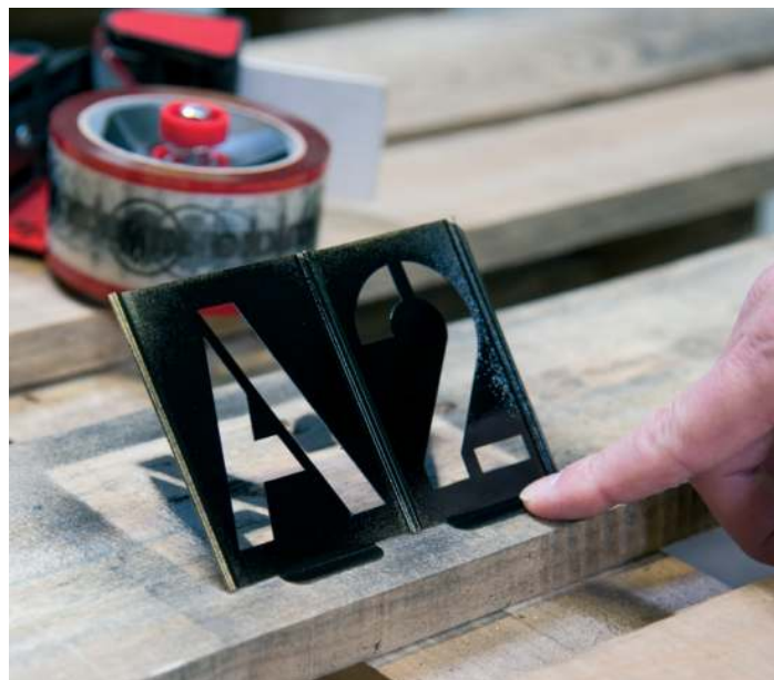
Marking stencils of series 327 in use
