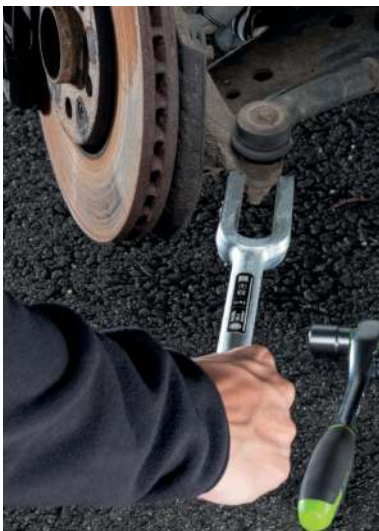
Separating a control arm from the wheel suspension
