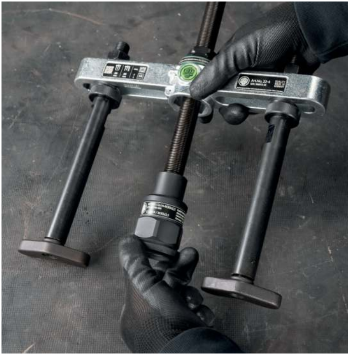
A thread adapter is combined with a counter stay (series 22) to disassemble a bolt with an external thread.
