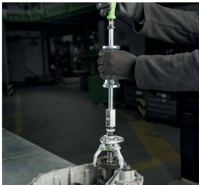
Disassembling a belt pulley from a transmission part
