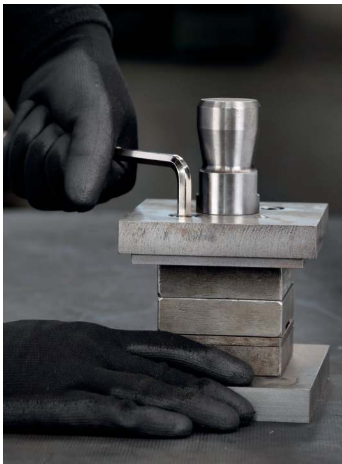
The allen keys from the SERIES 291 sales and workshop stand during the disassembly of a punching tool
