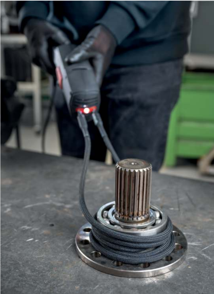
Heating a ball bearing with a flexible heating coil
