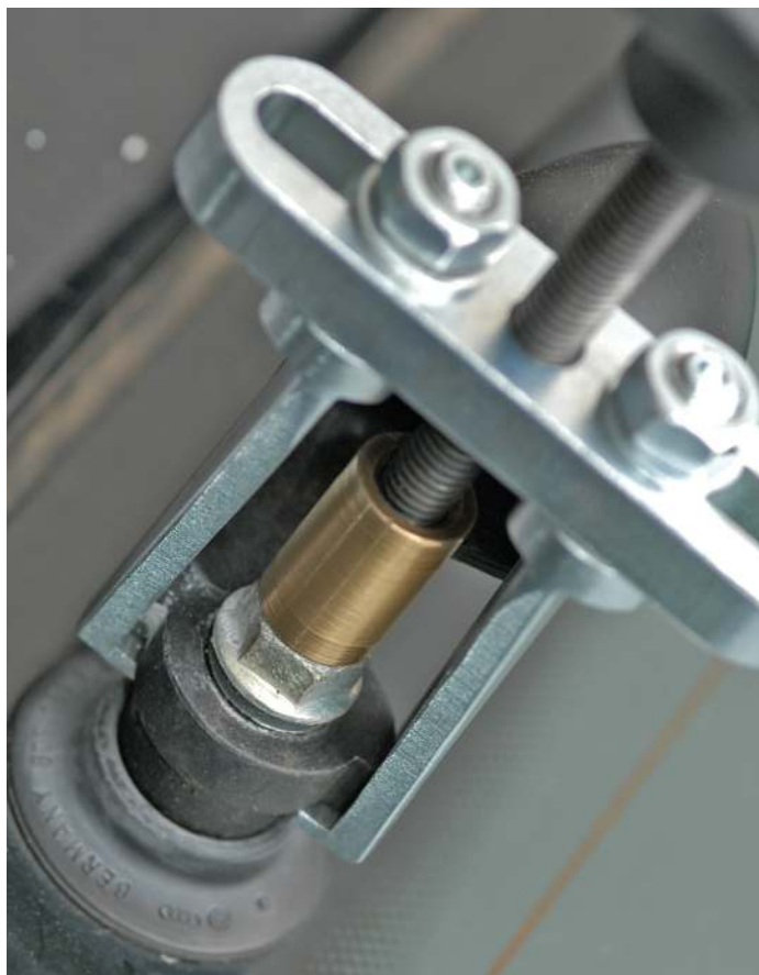
Removing a wiper arm with the 128-F-SW
