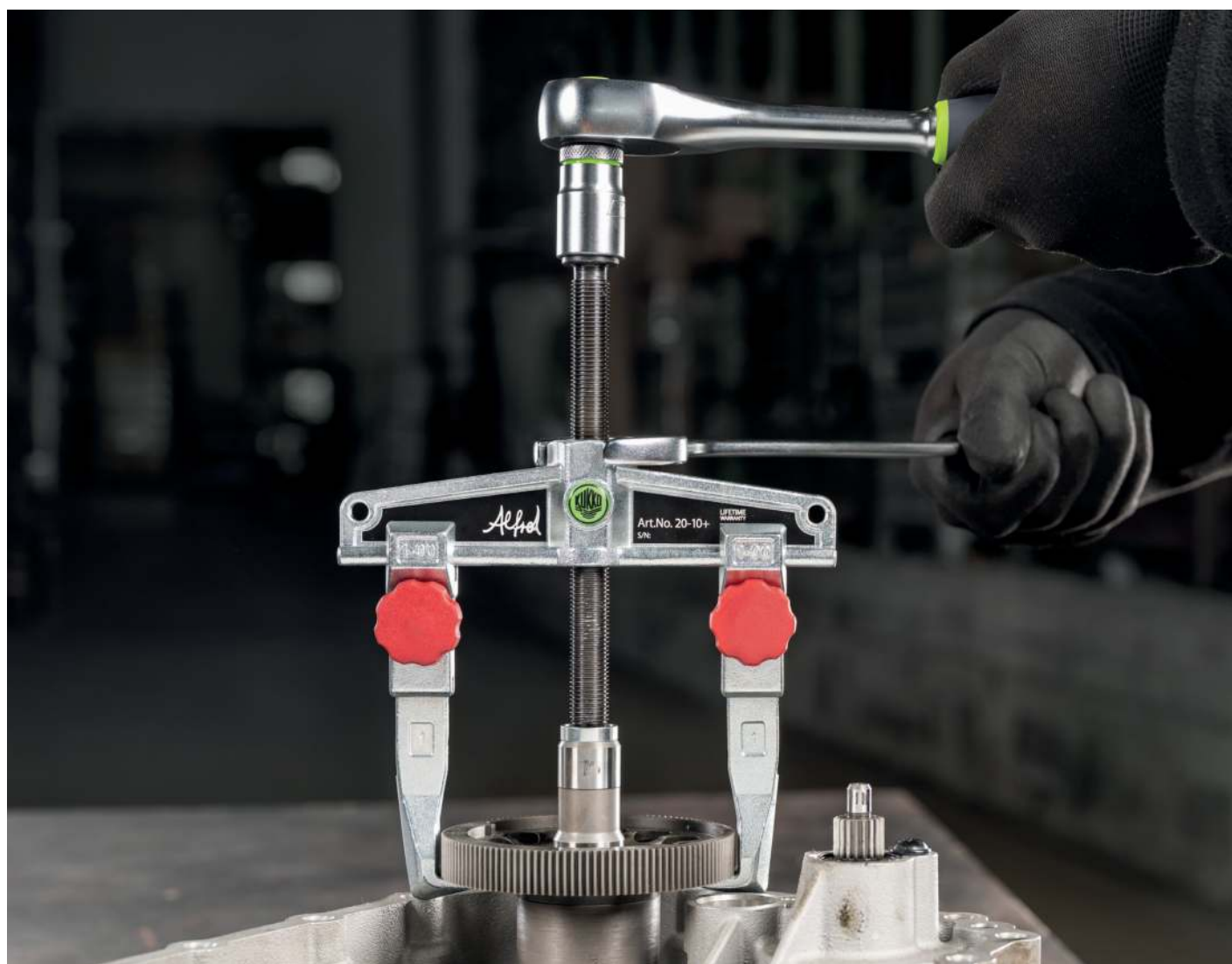
Pulling a transmission gear using the 20-10+
