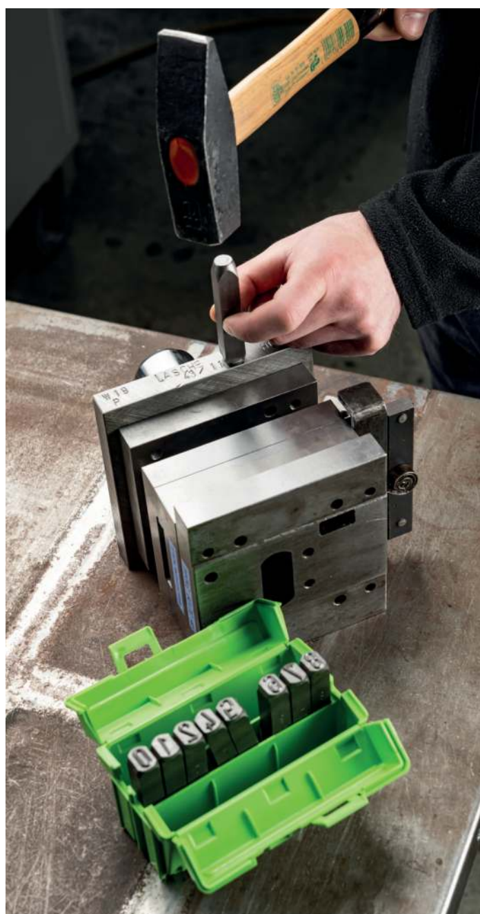
Marking a punching tool with number punches of series 328
