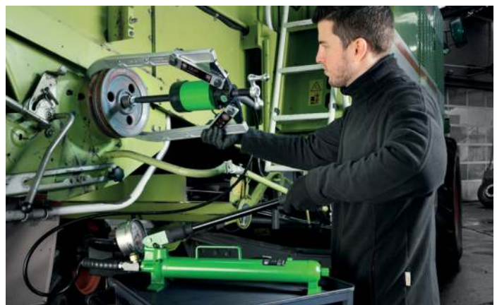
Pulling a pulley from a combine harvester with the Y28-205
