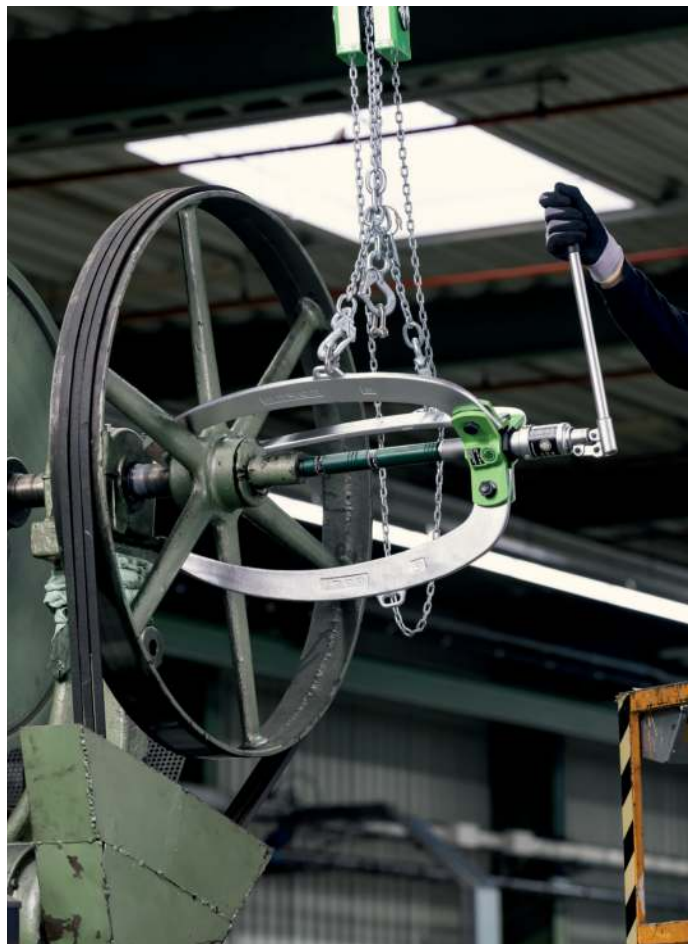
Pulling a pulley using the 45-8 with hydraulic spindle
