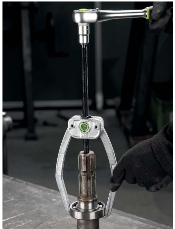
Removal of a ball bearing from a gear wheel
