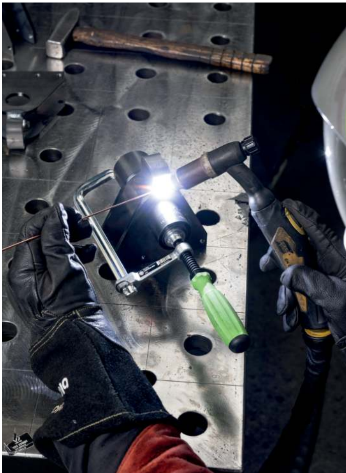
During welding work, the all-steel screw clamp acts as a "third hand." The picture shows a model from the 469P series.
