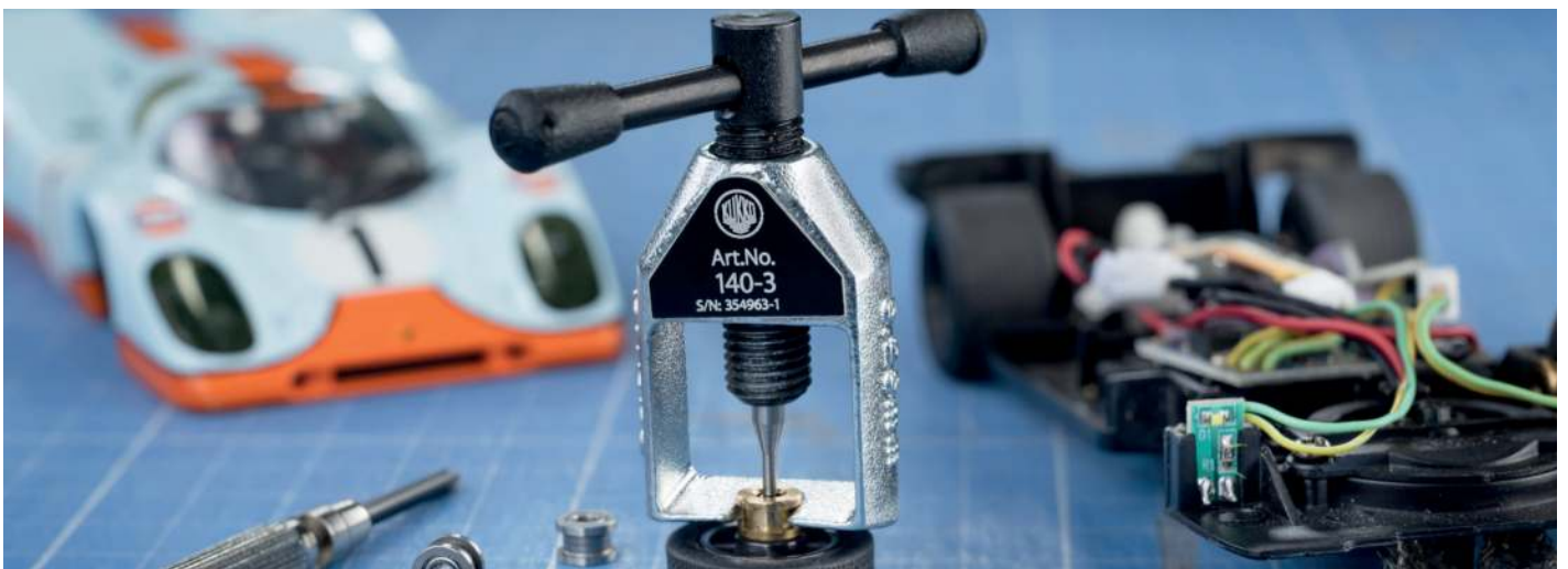
Removing a ball bearing from a model car tire with the 140-3
