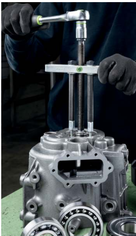
Ball bearing removal with the 69-A
