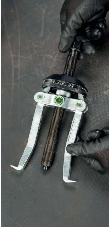
The internal extractor is ready for use
