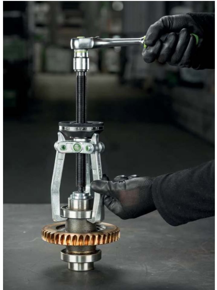
External extraction of a ball bearing from a gear shaft
