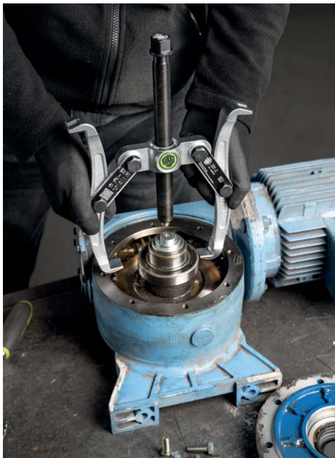
The oscillating jaws of series 201, 202 and 203 can be perfectly applied to the part to be pulled.
