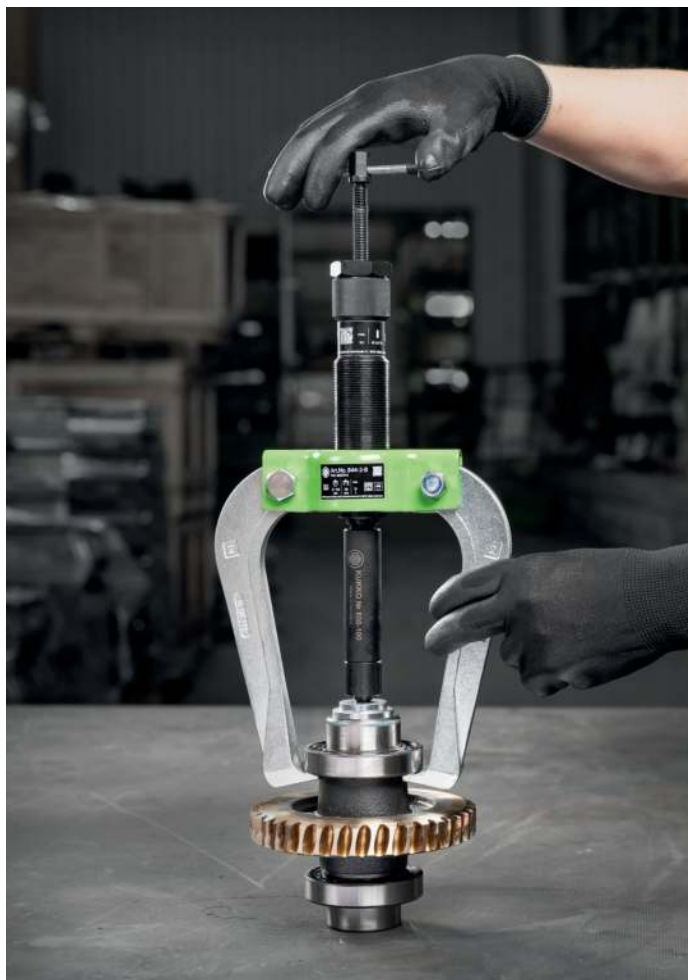
Pulling a ball bearing from the gear wheel
