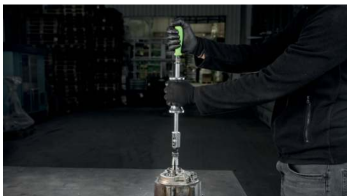
Extracting a ball bearing with sliding hammer and an internal extractor of series 21
