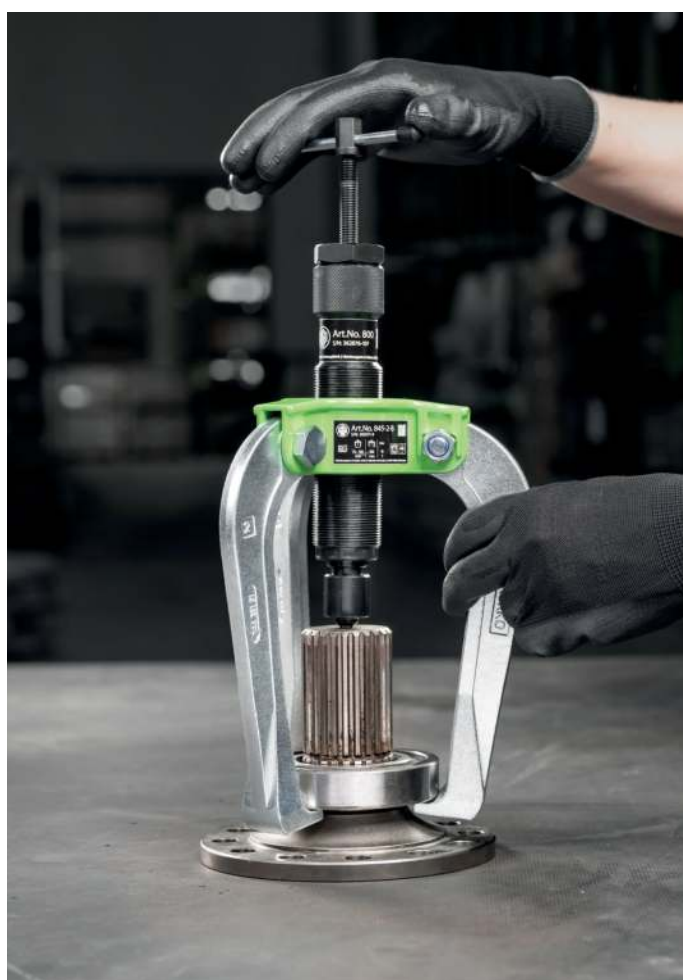
Removal of a ball bearing from drive flange
