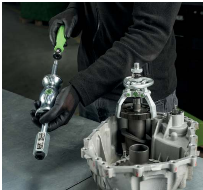
Attaching the 3-K handle G-22 to the sliding hammer
