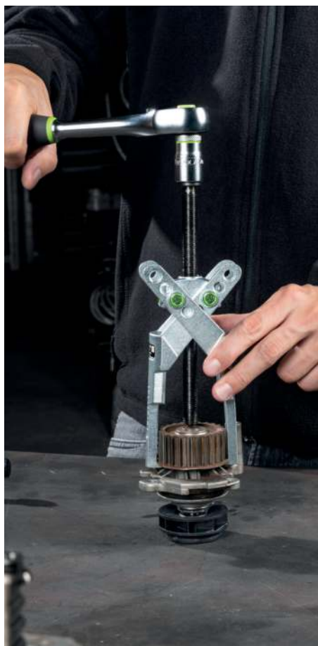
The scissor-like hook guide ensures a secure hold. The claw feet enclose the pulley
