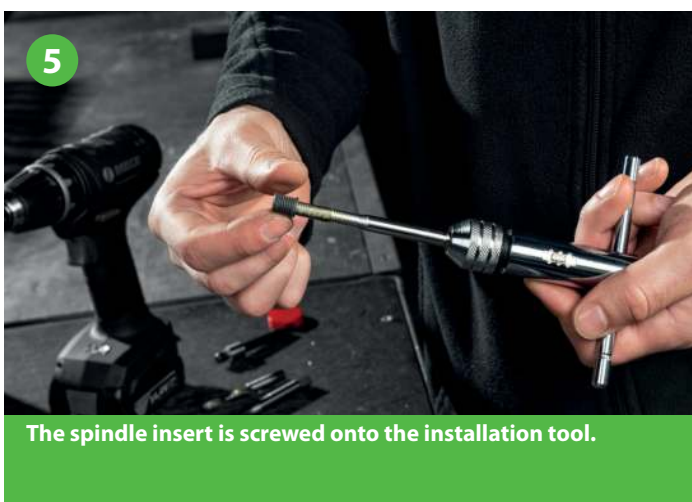
The installation tool screws in the spindle insert. The special shape of the installation tool also lightly presses the spindle insert into place.
