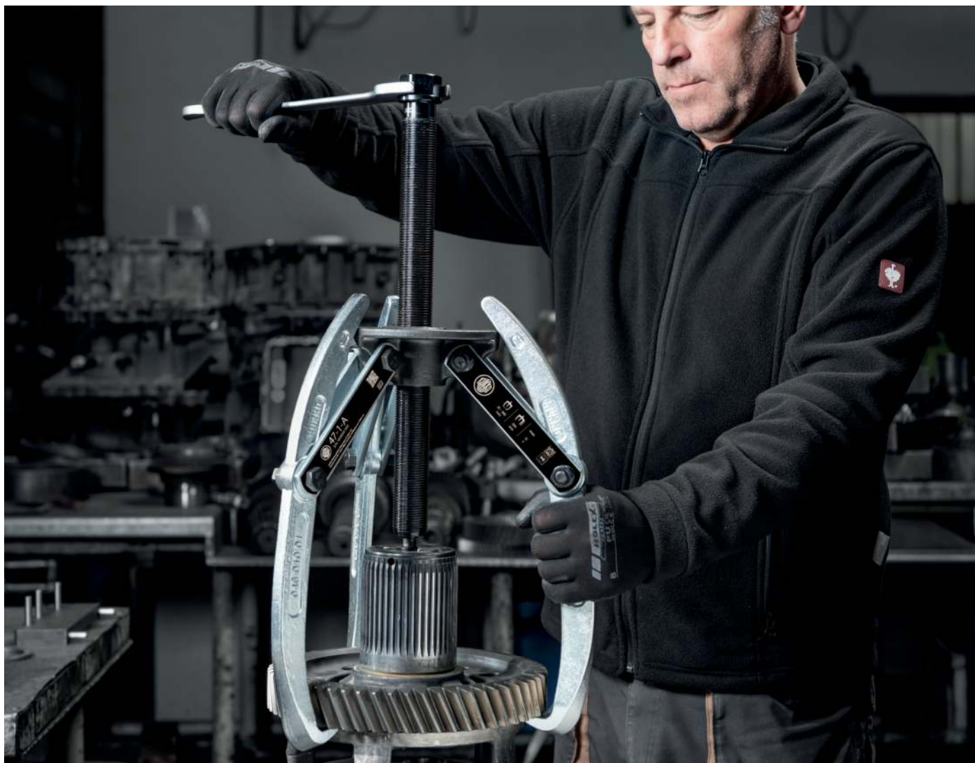
Pulling a gearwheel with the 47-1-A
