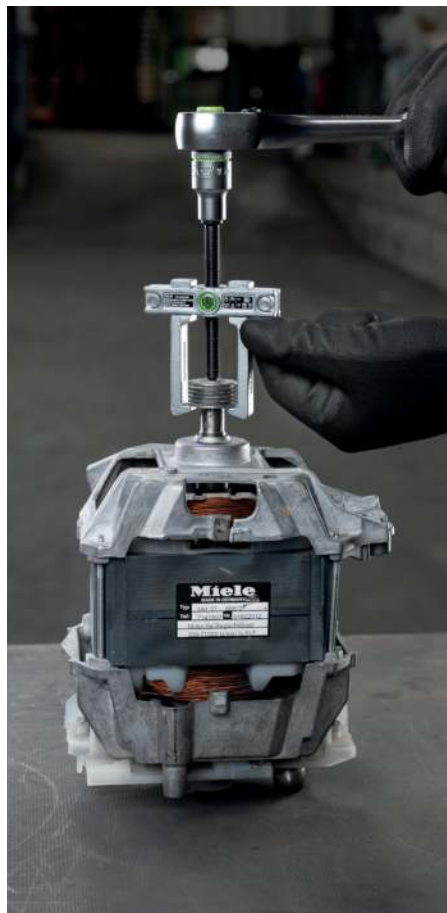
Pulling a pulley from a washing machine motor with the 110-01
