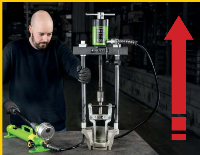
Disassembly of a cylindrical roller bearing with puller Y28-180, internal extractor Y-221-E and hand pump YHP-325
