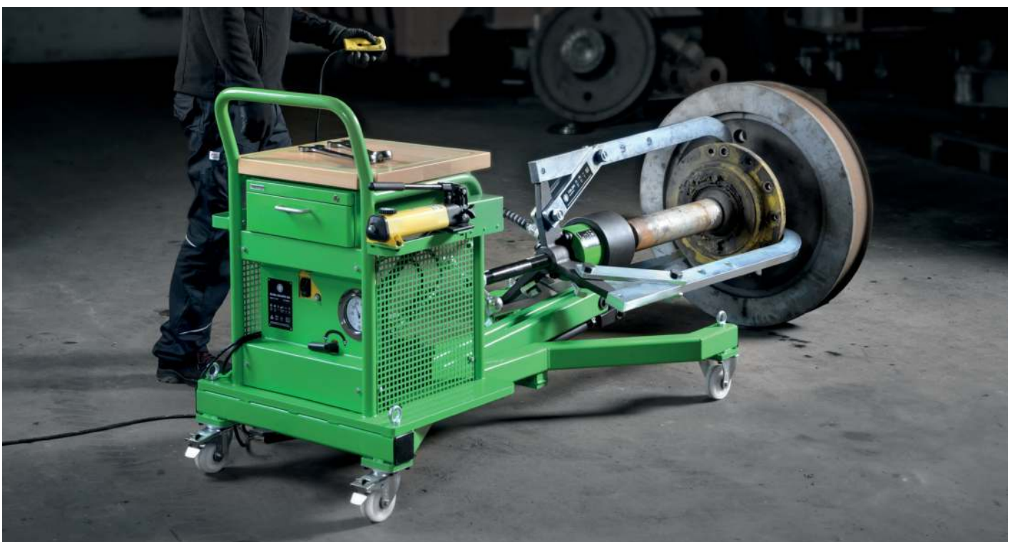
The mobile hydraulic puller “GOLIATH” Goliath-556 removing a tight-fitting wheel bearing from a harbor crane
