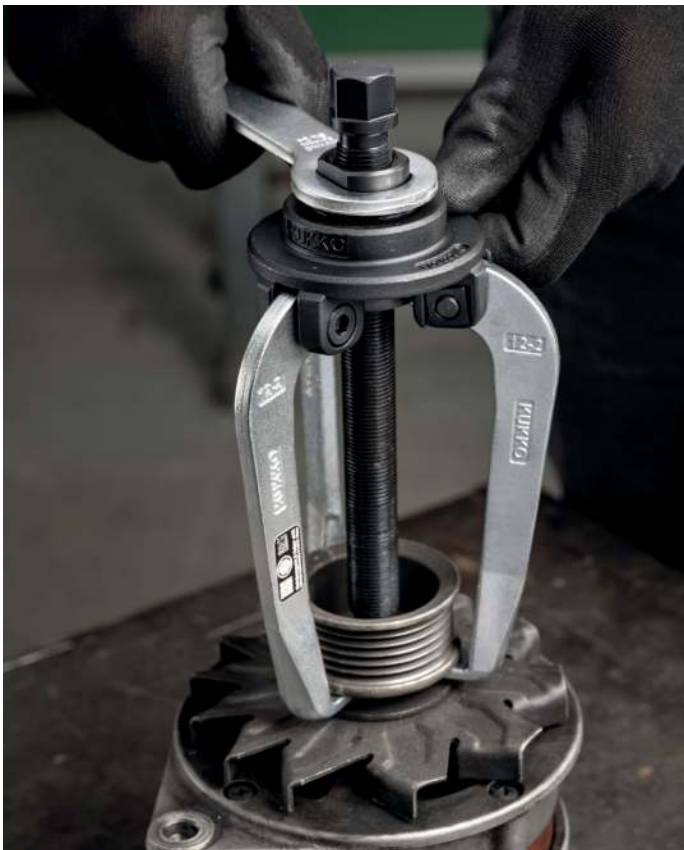
Removing a pulley from a car alternator
