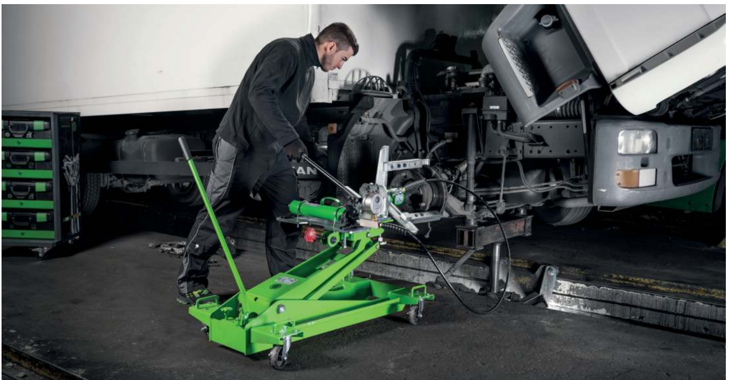
The mobile hydraulic puller “DAVID” in use
