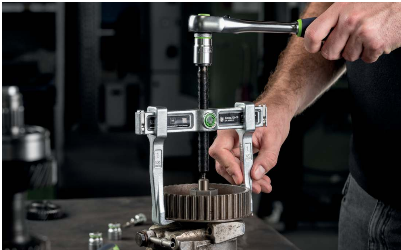
Pulling off a gear wheel with the 120-10
