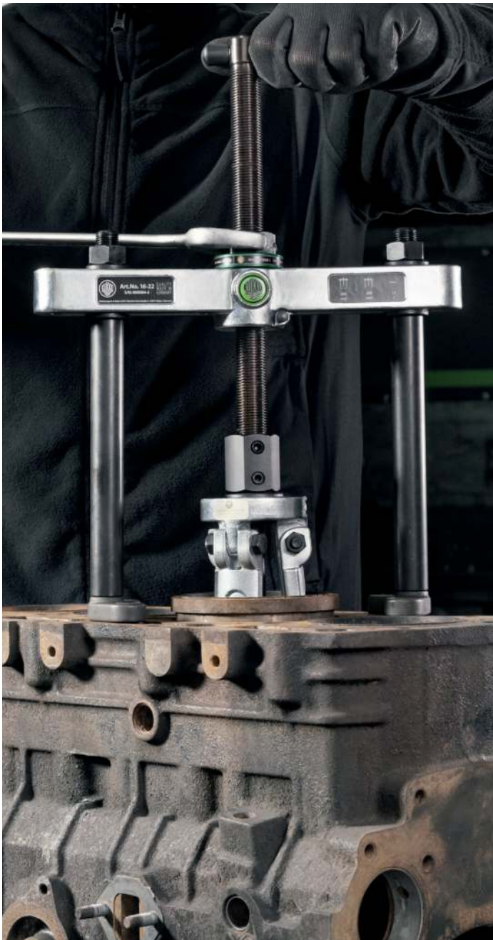
Extracting a cylinder sleeve with the 21-90 and the counter stay 22-5
