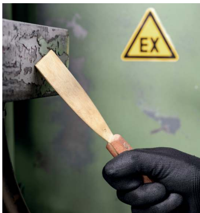
Non-Sparking spatula in use on metal surface
