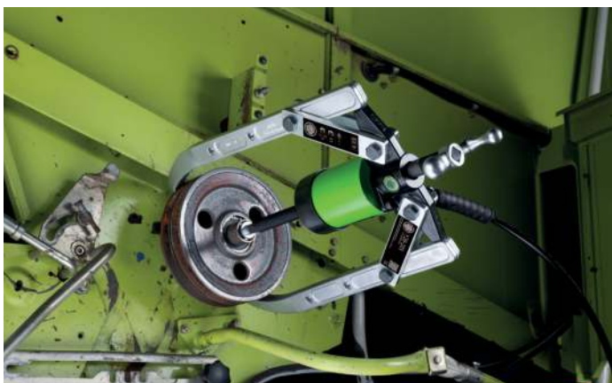
Pulling a pulley from a combine harvester with the Y28-205
