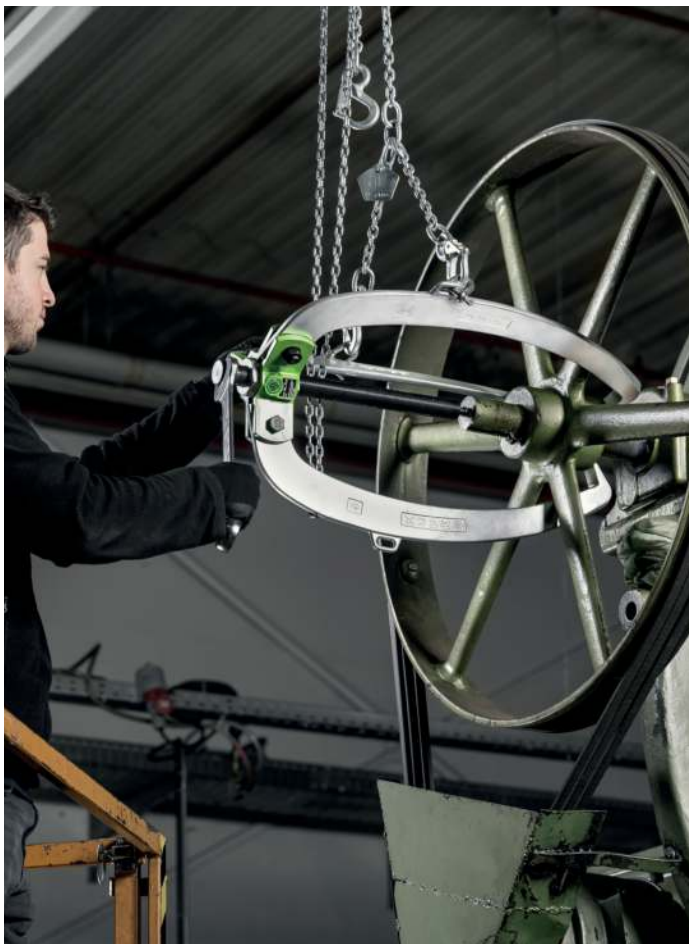
Pulling a pulley using the 45-8 with a mechanical spindle. For locking and holding, the Puller is attached to the URANUS.
