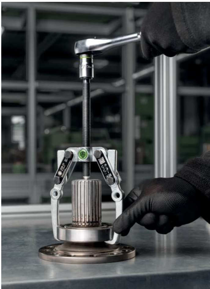
Pulling a ball bearing from a shaft with the 208-01.
