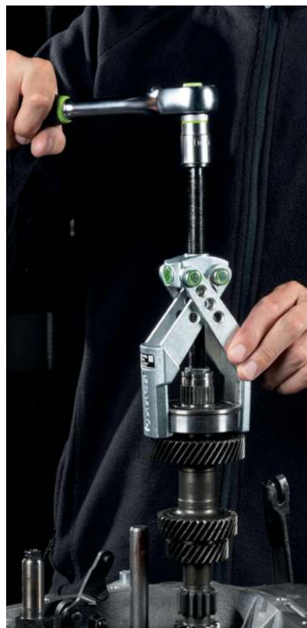
Pulling a ball bearing from a gear shaft
