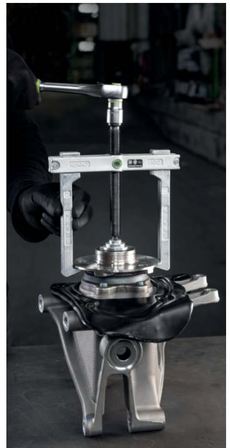
Pulling a wheel hub from a steering knuckle with the 110-2
