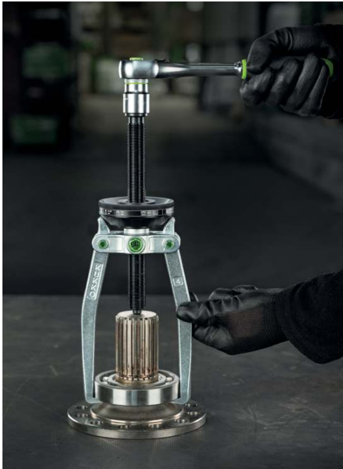
External extraction of a ball bearing from a drive shaft
