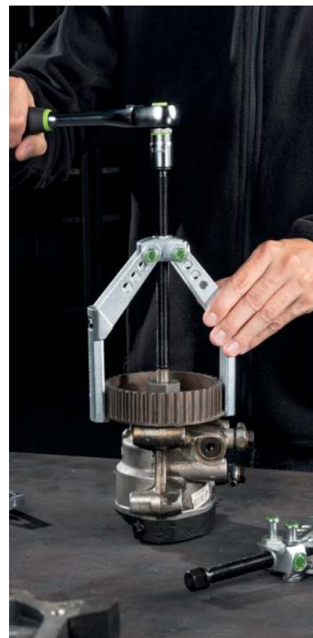
The crossover of the jaws increases the span range many times over
