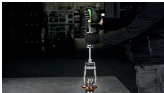
Pulling a ball bearing with a sliding hammer and the puller 220-2
