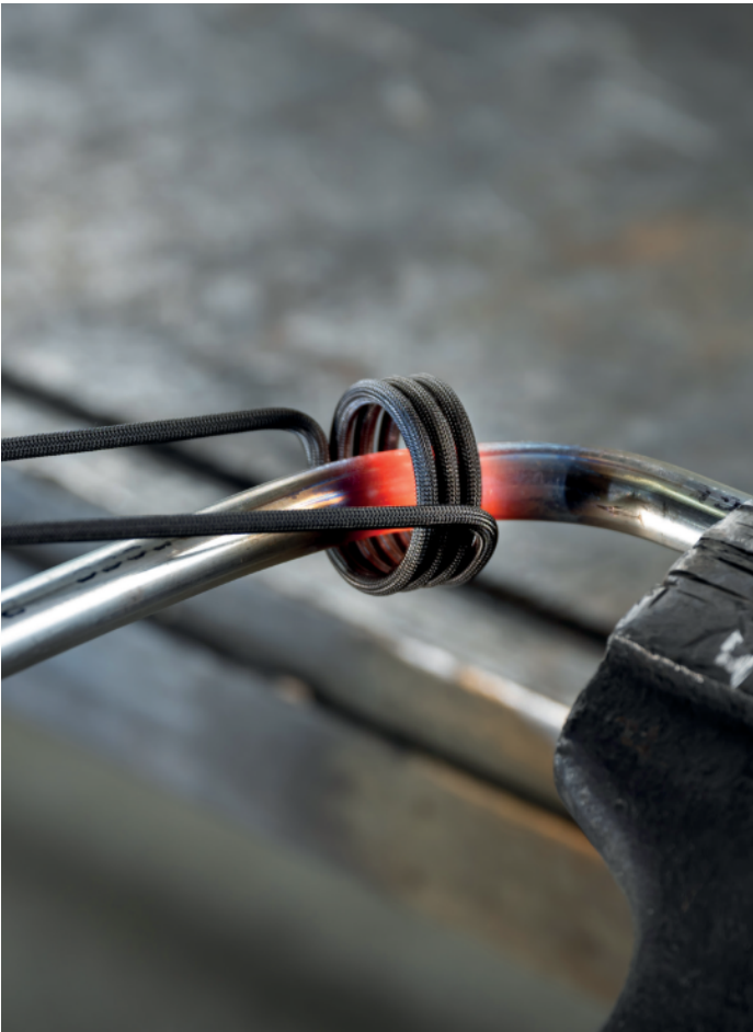
Heating a pipe with a heating coil to bend it afterwards
