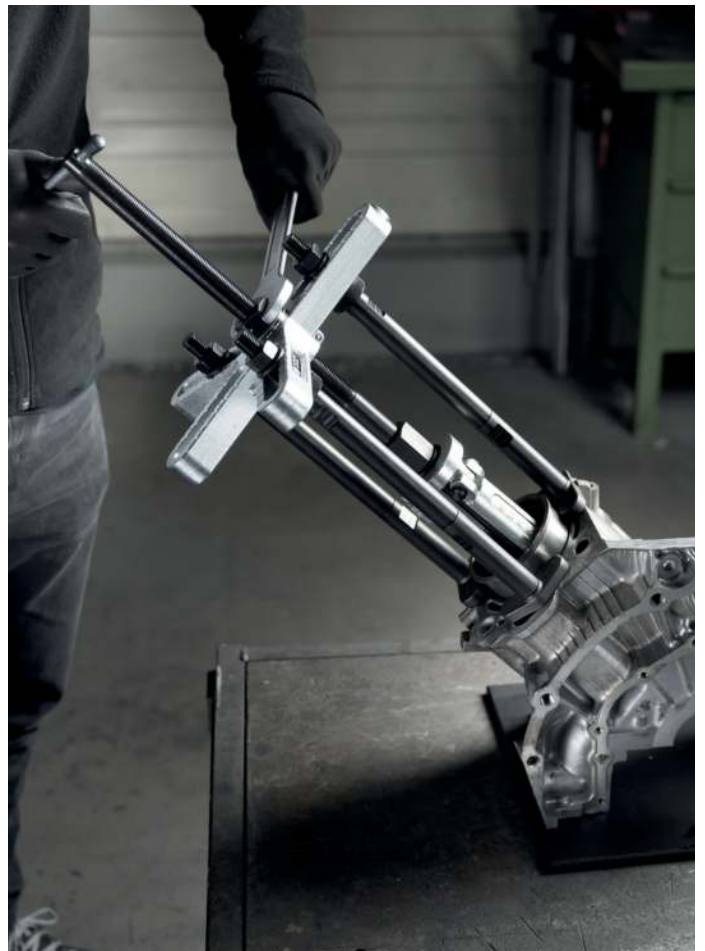
With three foot bolts on the multi-crossbar you achieve optimal positioning during the extraction process using the 16-2 cylinder liner puller
