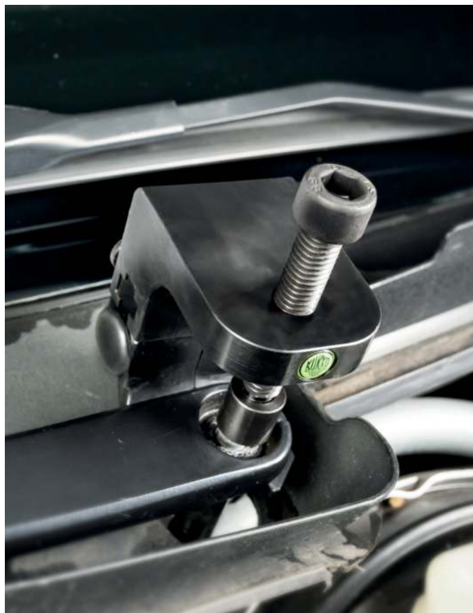
Removing a wiper arm with the 128-F-60
