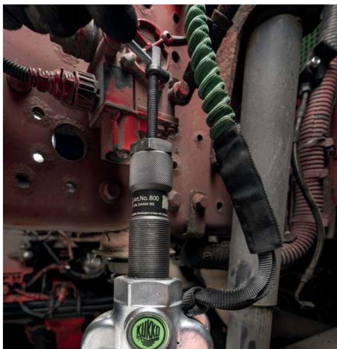
Fall protection secures ball joint puller
