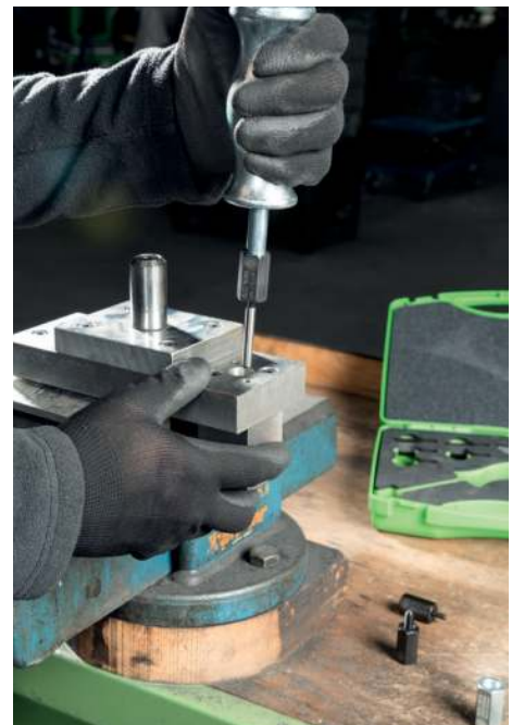
Extracting a dowel pin using a sliding hammer and thread adapter
