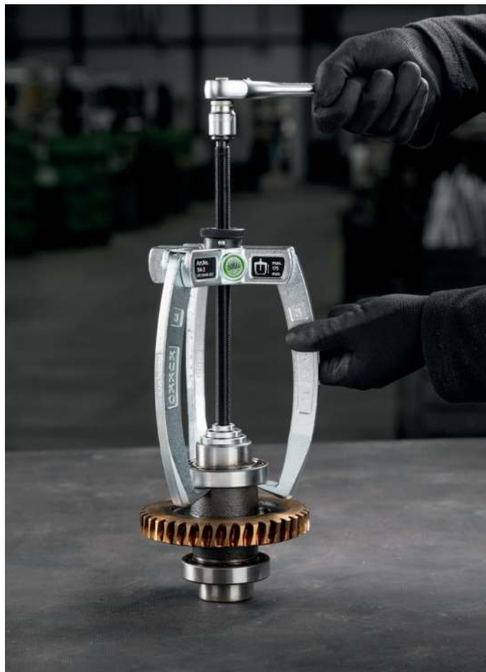
The 3-jaw Kombi-Puller of Series 114 during external extraction of a ball bearing from a gearbox component
