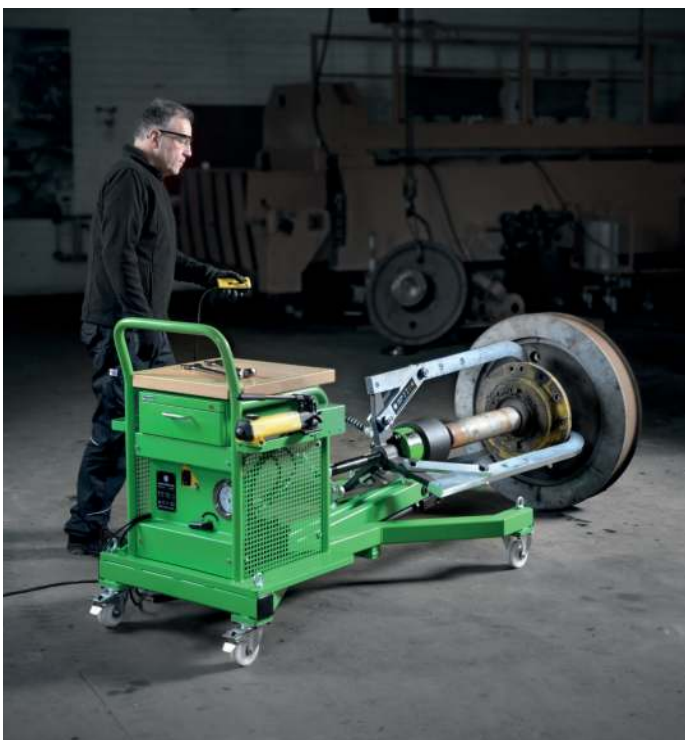
The mobile hydraulic puller “GOLIATH” Goliath-556 when extracting a seized wheel bearing from a harbour crane
