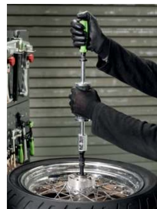
Internal extractor of series 21-E with sliding hammer
