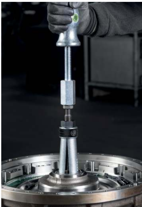
Extracting a ball bearing using a sliding hammer, connecting nut and thread adapter
