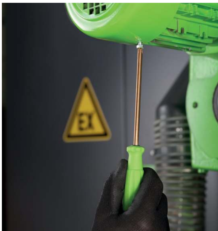
Unscrewing a screw using a Non-Sparking screwdriver
