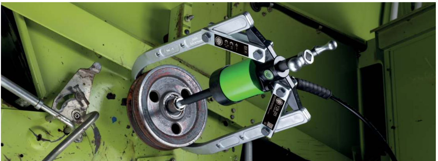
The hydraulic puller Y28-205 was mounted on the pulley and is ready for use
