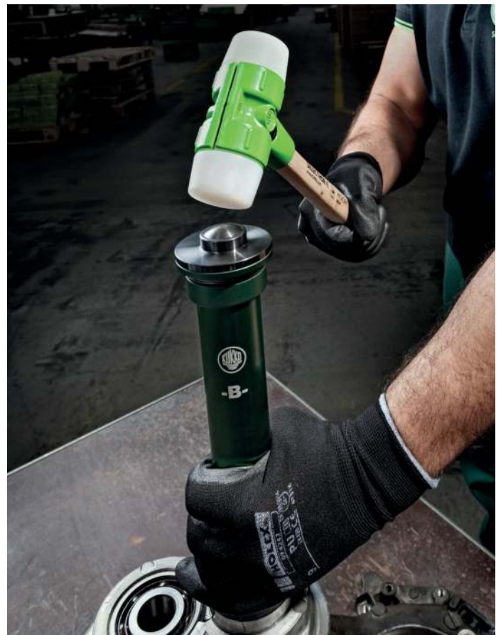
Installation of a gearbox bearing with a Selecthor soft-face hammer in combination with the 71-L
