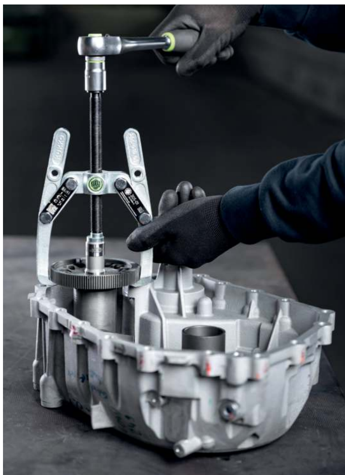
Removing a transmission gear using the 205-01
