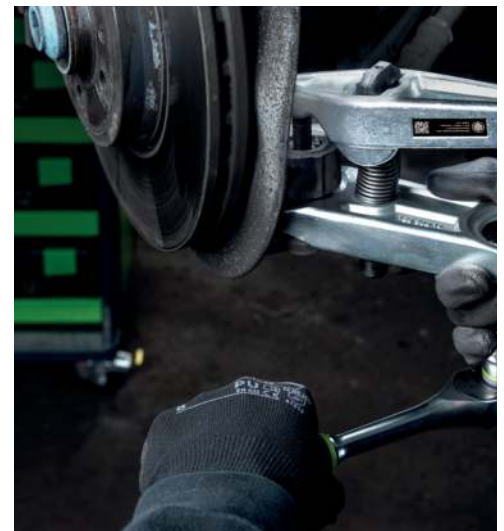
The ball joint press 129-3 in use pressing out a tie rod end in a workshop
