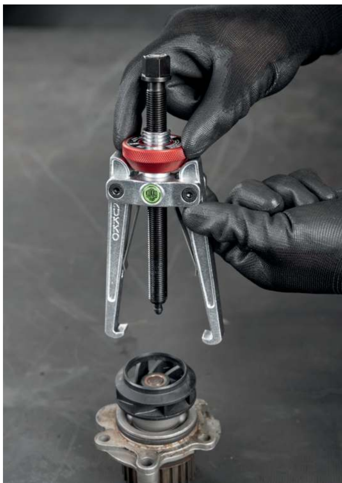
The 2-jaw Puller for roller bearings 112-20 with cone knob when removing a ball bearing on a water pump
