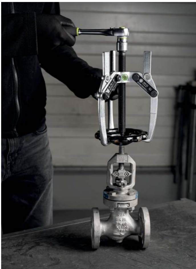
Pulling the hand wheel from a shut-off valve with the 209-02.
