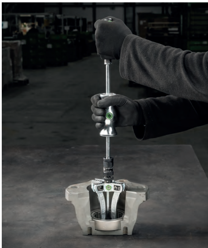
3-jaw internal extractor (114-2) with slide hammer when extracting a cylindrical roller bearing from a housing
